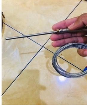
Gambar 4.13. Sensor thermocouple tipe K
