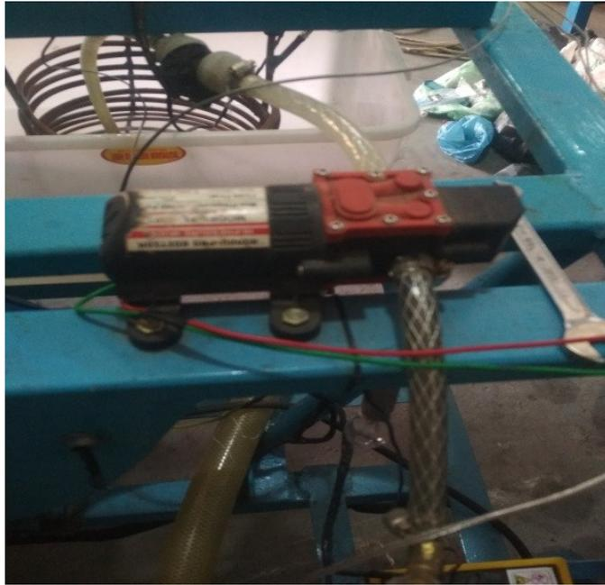
Gambar 3.15 Pompa Air Elektrik High Preasure 12v
