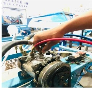
Gambar 4.19. Memasang selang manifold
