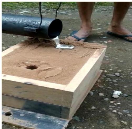
Gambar 3.19. Menuang Cairan Alumunium
