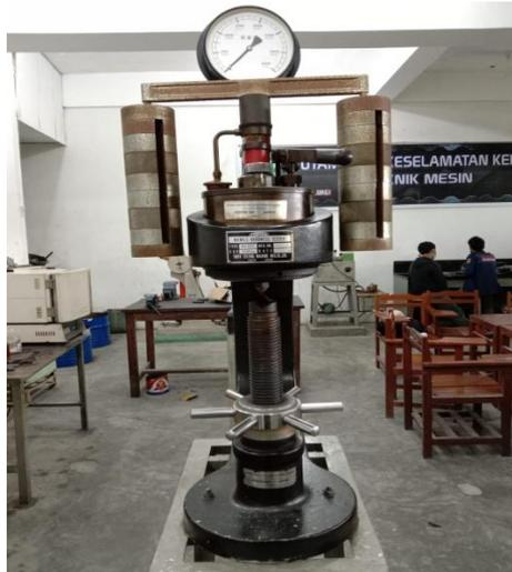
Gambar 3.22. Brinell Hardness Tester
