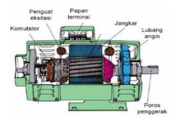
Gambar 2.5 Generator Arus Searah (DC)
