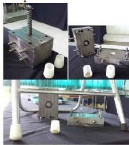
Gambar 2.2. cetakan ( mould ) (Hadi et al., 2015)
