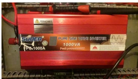
Gambar 2.3 *Inverter pure sine wave*
