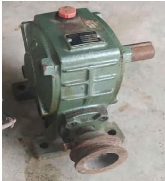
Gambar 3.5 Gearbox/transmisi
