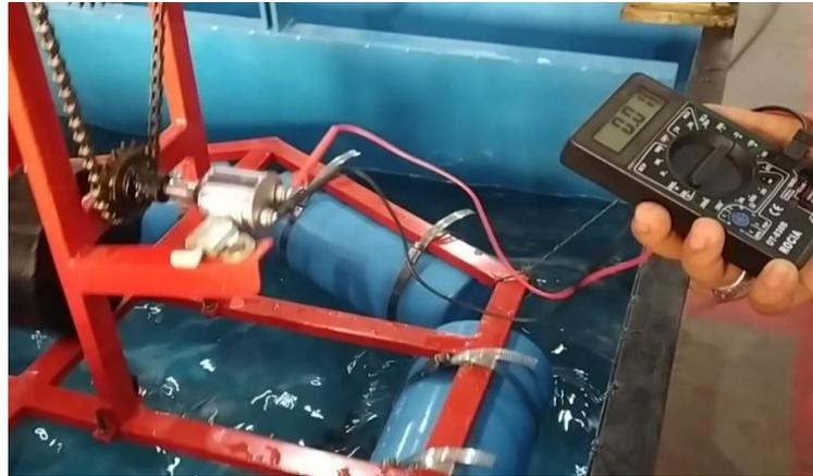
Gambar 4.20 Mengukur arus
