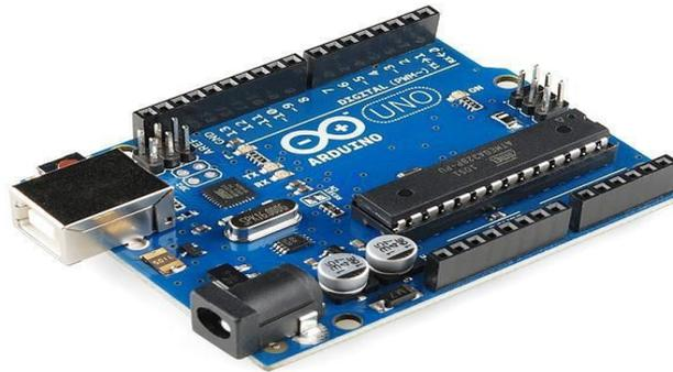
Gambar 2.4 Board Mikrokontroler ATmega328
