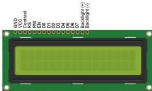
Gambar 2.15 LCD 16 x 2
