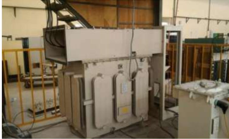
**Gambar 3.1** Induction voltage regulator
