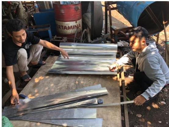
Gambar 3.20 Memotong Plat Alumunium
