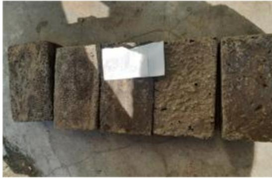
Gambar 4.7 paving block campuran botol plastik 70% dan pasir 30%
