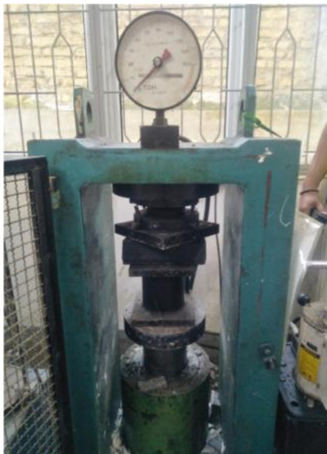
Gambar 4.8 Mesin Compression test
