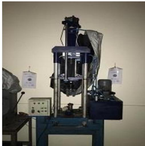
Gambar. 3.15 Alat Uji *Three Point Bending*
