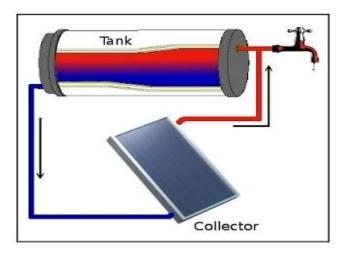
Gambar 2.2 Solar Water Heater Pasif
