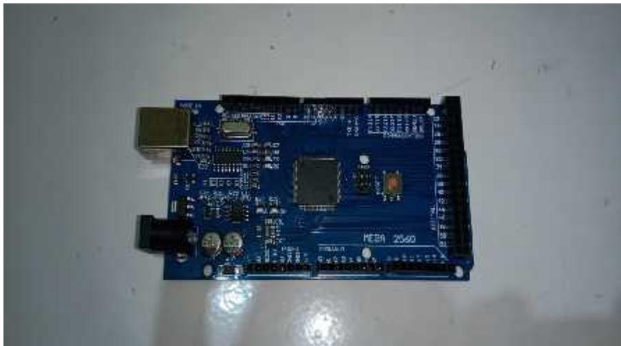
Gambar 3.1 Arduino ATmega2560
