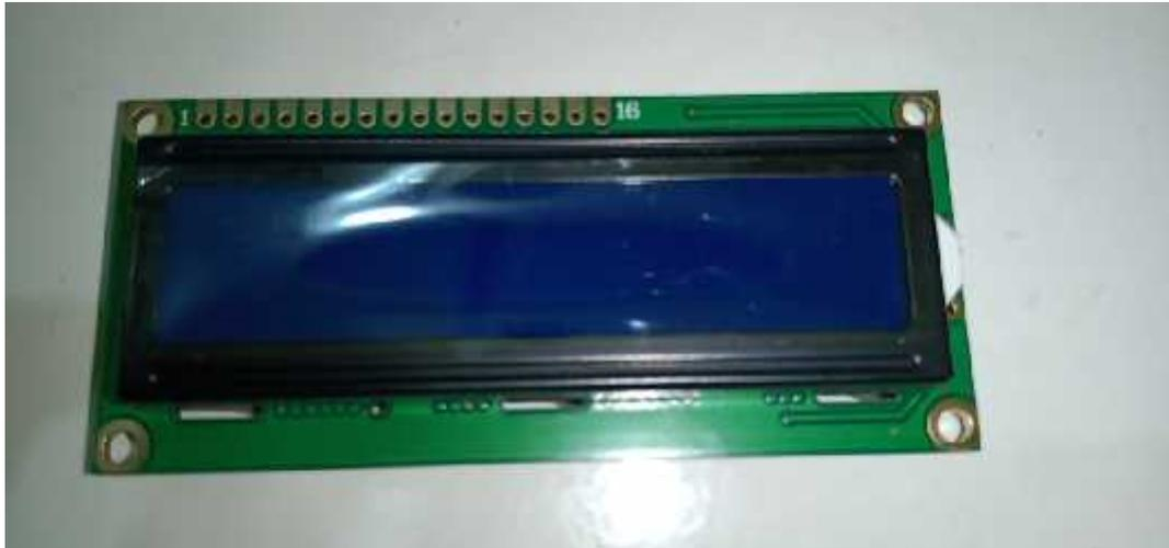
Gambar 3.7 LCD 16x12
