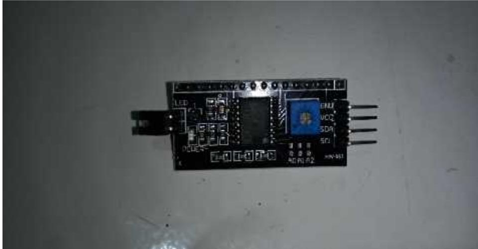
Gambar 3.3 12C Serial Interface Board
