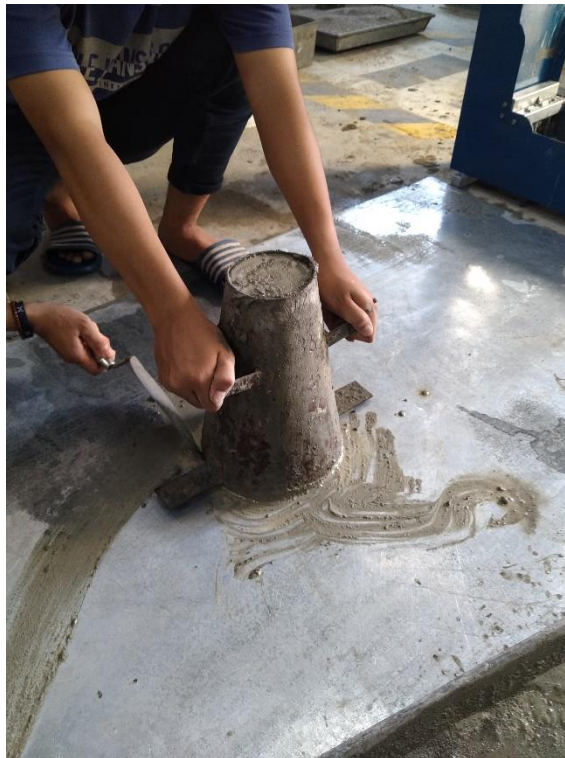
Gambar 3.3: Pengujian Slump Flow .
