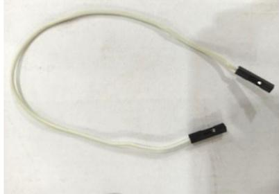
Gambar 2.20 Kabel Female to Famale
