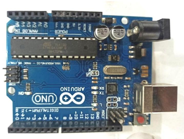
Gambar 2.32 Board Arduino Uno R3
