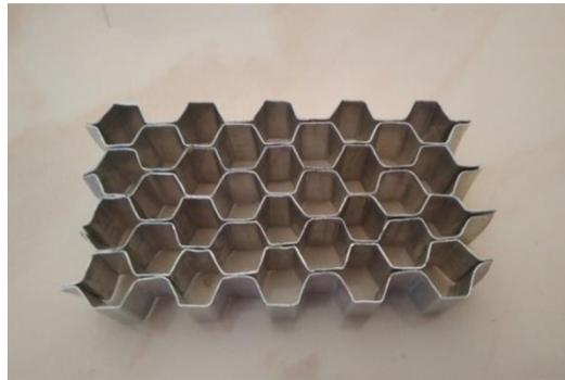
Gambar 4.8: Spesimen ukuran hexagonal 6 mm
