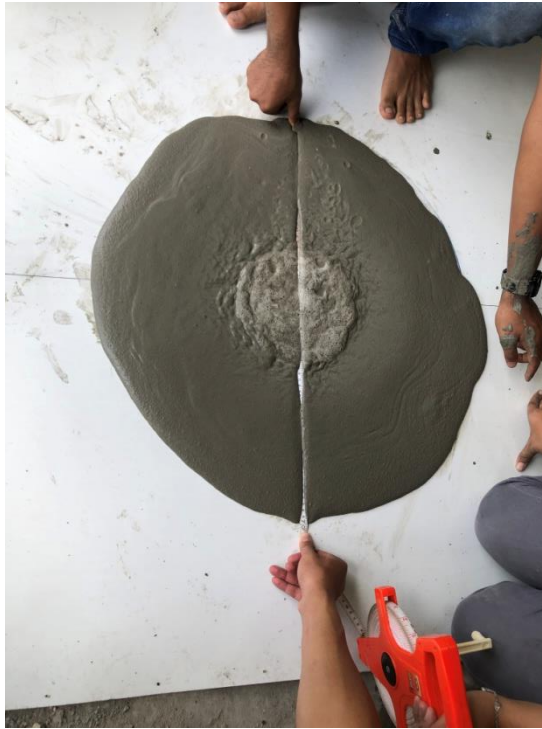
Gambar L11. Mengukur diameter slump flow
