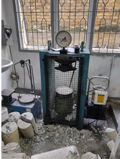
Gambar L.1: *Compressing Test Machine.*
