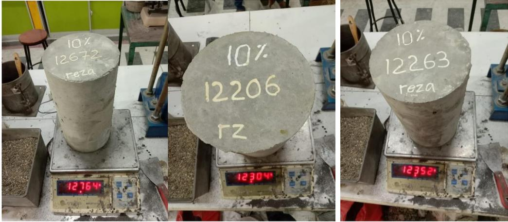
Gambar L.25: Beton abu cangkang -10%.
