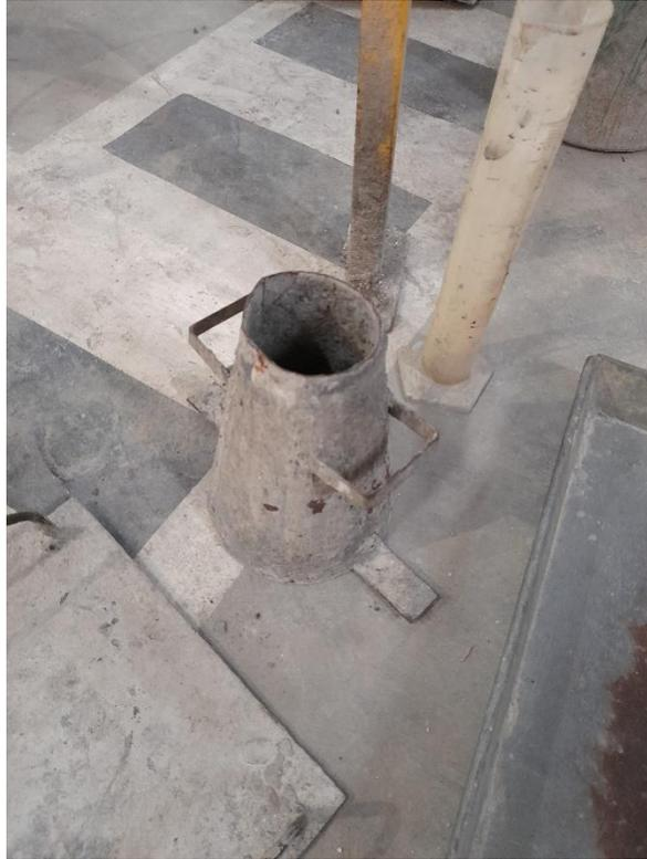
Gambar L.7: Kerucut Abrams.
