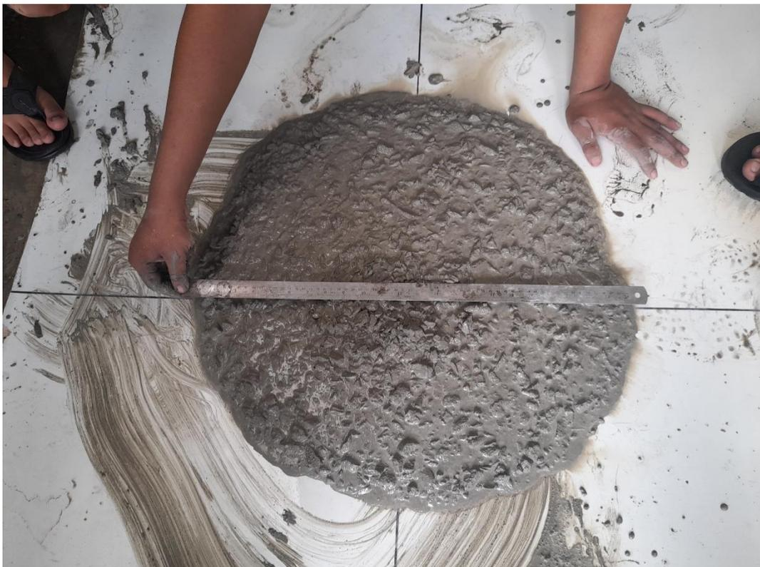
Gambar L.20: Pengukuran diameter *slump flow*.
