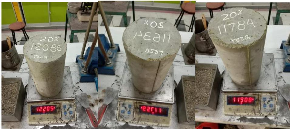
Gambar L.28: Beton abu cangkang 20%.
