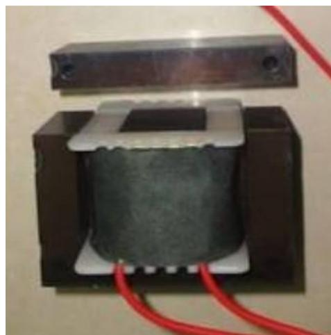
Gambar 2.13 Elektromagnet (*Vibrator coil*)
