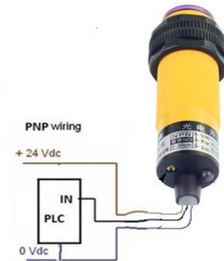
Gambar 3.2 Wiring Sensor *Photoelectric*
