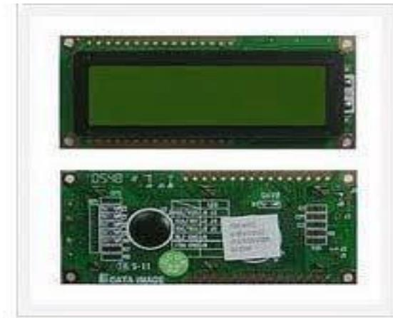
Gambar 2.8 Liquid Crystal Display LCD
