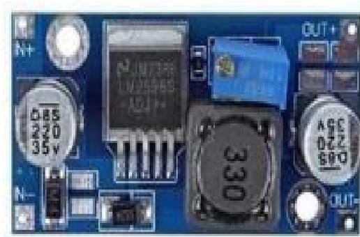
Gambar 2.9 Modul Buck Converter
