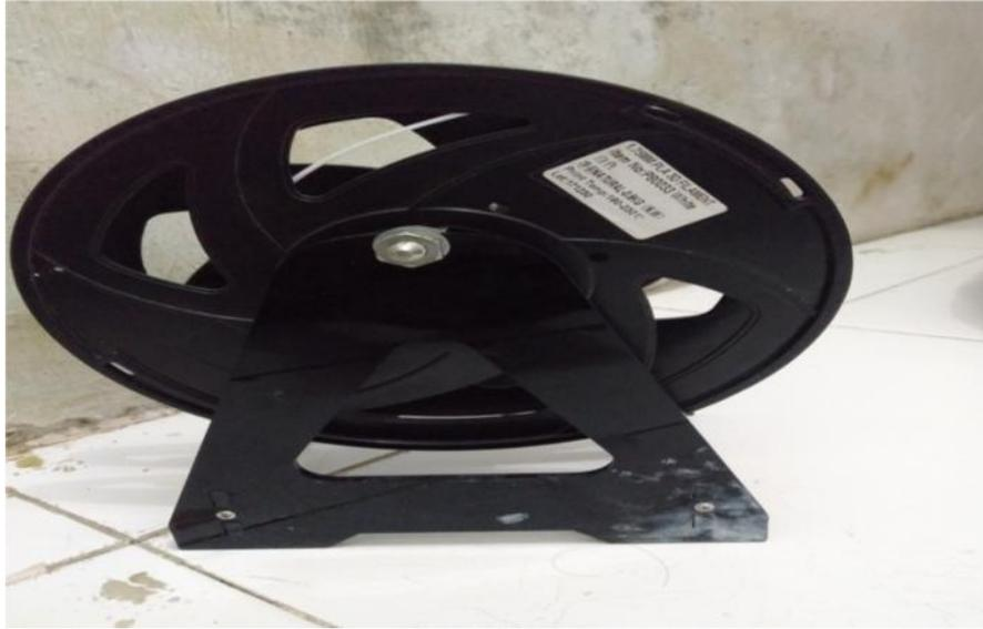
Gambar 3.9 filament pla 3D printer
