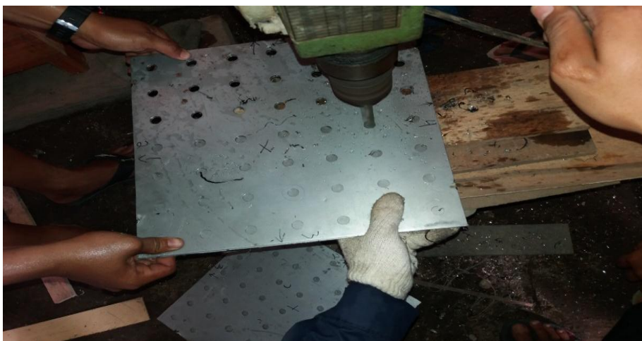
Gambar 3.26 Melubangi plat besi (350 mm x 350 mm)
