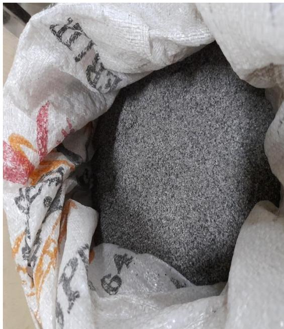
Gambar L- 20 : Abu Cangkang Kelapa Sawit
