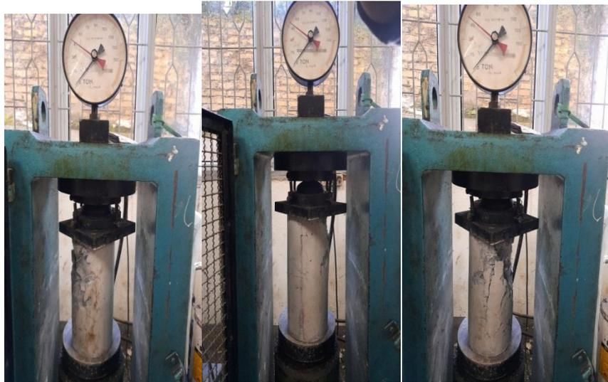
Gambar L- 33 : Nilai Kuat Beton Normal
