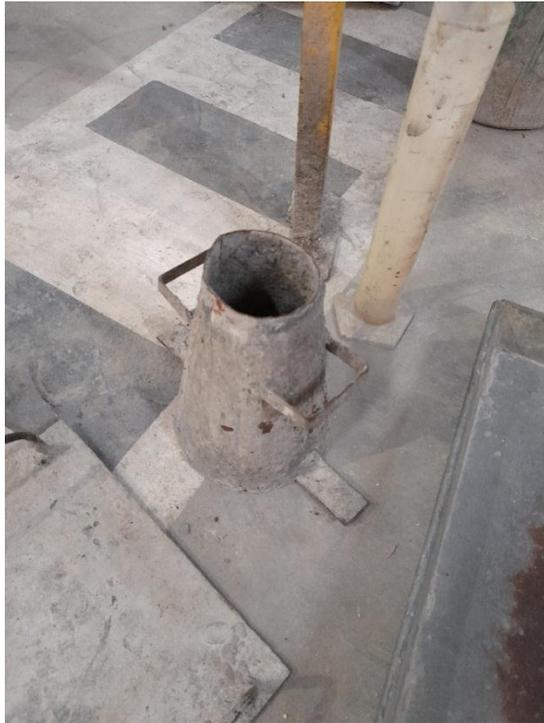
Gambar L- 7 : Kerucut Abrams
