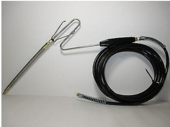
Gambar 3.7. Exhaust Probe
