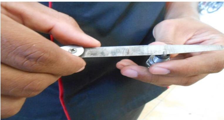
Gambar 3.2: Celah elektroda busi standard ngk c7hsa (0.7 mm)
