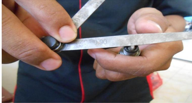
Gambar 3.3: Celah elektroda busi renggang ngk c7hsa (0.9 mm)
