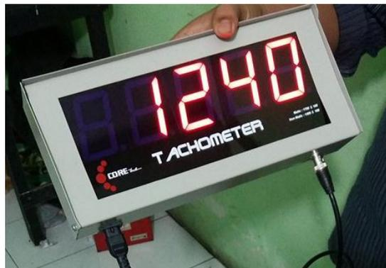
Gambar 3.3 Alat Tachometer
