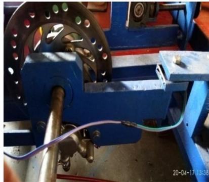
Gambar 3.7 Sensor Loadcell
