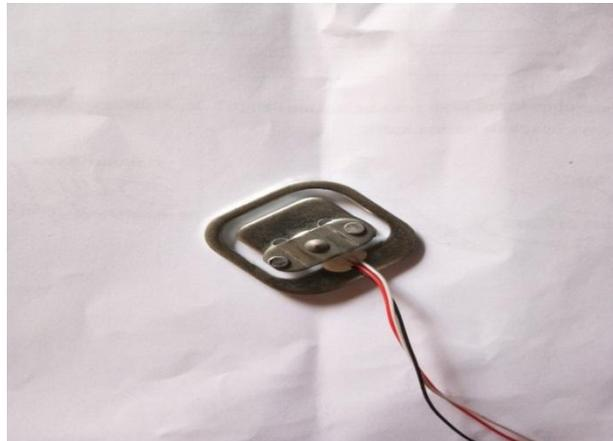
**Gambar 3.10.** Sensor *Load Cell*
