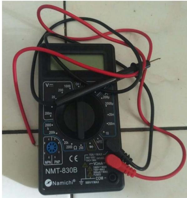
**Gambar 3.5 Multimeter**
