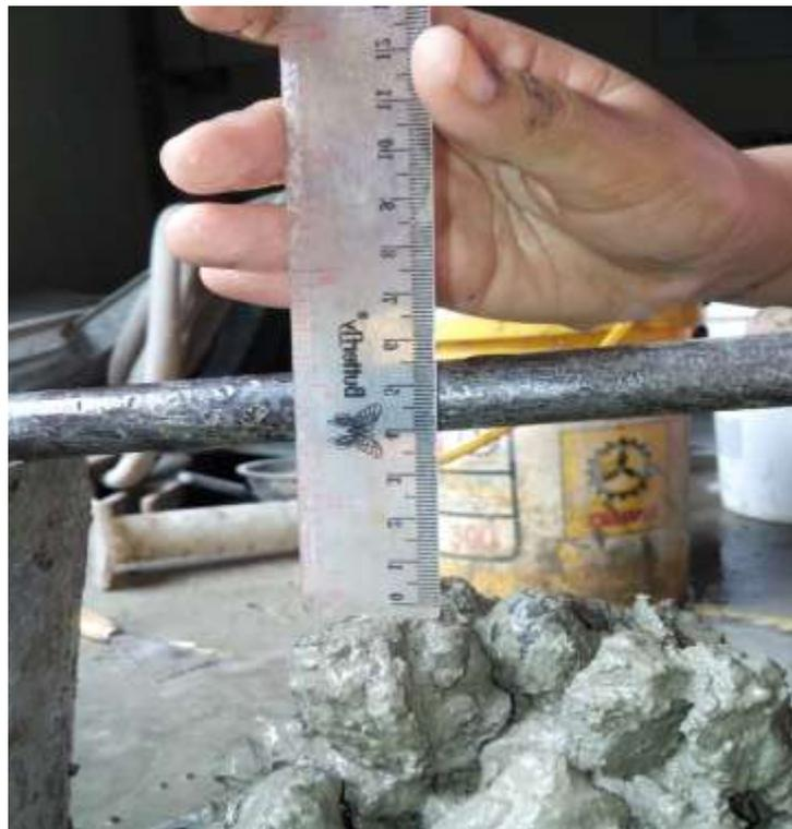
Gambar L6: Hasil pengujian slump test.
