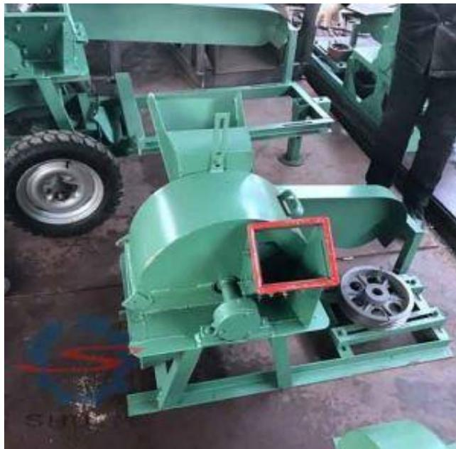
Gambar 2.2. Mesin Penghancur kayu (Sumber:[https://id.thereshermachine.net/charcoal-briquette/wood-crusher-machine mesin-penghancur kayu](https://id.thereshermachine.net/charcoal-briquette/wood-crusher-machine-mesin-penghancur-kayu)).
