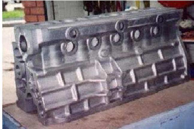
Gambar 2.7. Blok Silinder Hasil *Sand Casting*
