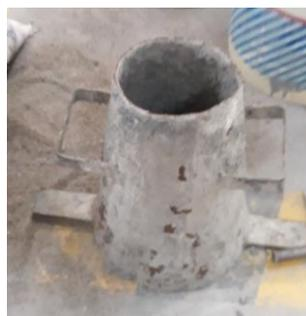
Gambar 3.14: Kerucut abrams.
