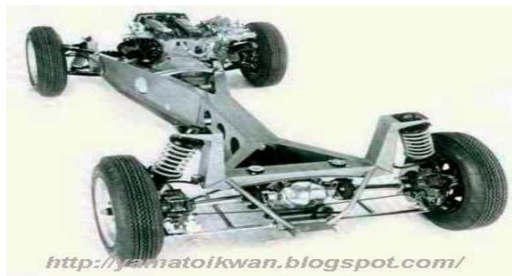
Gambar 2.4. Chassis jenis backbone
